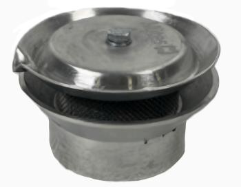
Vacuum Vent Caps are installed on the top of vent pipes from underground or above ground fuel storage tanks. The vent cap is designed to protect the tank vent lines against intrusion and blockage from water, debris or insects. The vent cap is designed from an aluminum body.
