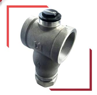
When there is a fuel overflow in the breath line to which the stainless steel ball inside is connected, it rises along with the liquid and seats itself in its socket, preventing fuel transfer to other tanks. It continues to allow vapor passage.
