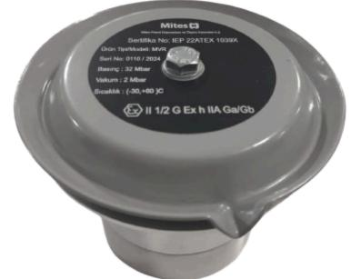
Pressure Vacuum Vents are installed on the top of vent pipes from underground or above ground fuel storage tanks. The vent cap and internal wire screen are designed to protect the tank vent lines against intrusion and blockage from water, debris or insects. A normally closed poppet in the valve opens at a predetermined pressure or vacuum setting to allow the tank to vent.
